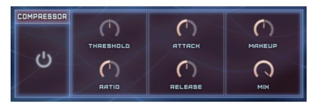
This Compressor is modelled on a classic analog bus compressor. It offers a more characteristic dynamic control than a standard compressor.
