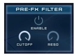
Cutoff - Set the frequency above which the sound is attenuated by the filter
