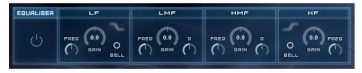
This EQ is modelled on high quality analogue circuitry. It is a 4-band parametric EQ and offers the choice of bell or shelf style control of the low and high frequency bands.
