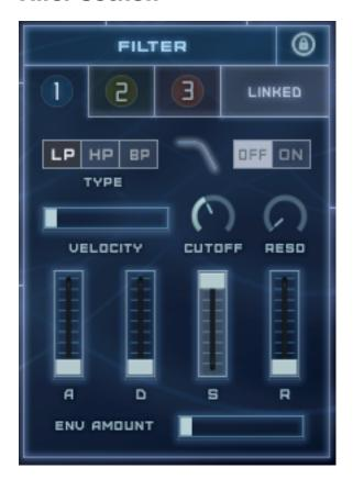
With this section you can apply a High Pass, Band Pass or Low Pass filter to each (or all) layers and adjust various parameters and the envelope relating to the filter.
