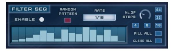
This allows you to apply the filter to create a Rhythm through the pattern in the table. A full step will not apply any filter, whereas an empty step will fully apply the filter, with anything in between applying the filter to varying degrees.
