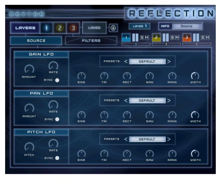
This section is accessed by clicking the Rhythm tab at the bottom and then the 'Source' button at the top. It contains 3 Low Frequency Oscillators (LFO's) that can be applied to the original sample to create Rhythm's & Pulses. It does so by generating periodic (or in some cases, random) signals, which are applied to the sound. Since version 1.6, each layer can have it's own unique LFO or they can be linked so they are all the same.
