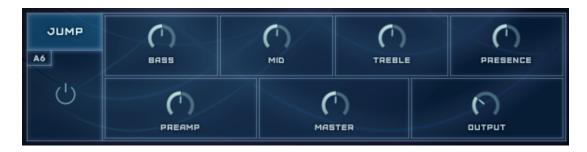
This effect simulates the classic tone of British guitar amplifiers. Be wary, this effects causes extreme distortion and loud levels so use with caution - start with the output turned low!
